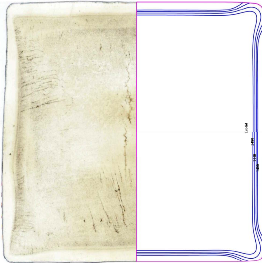
Fig. 27: Calculated temperatures in transverse billet section compared with measured shell shape
